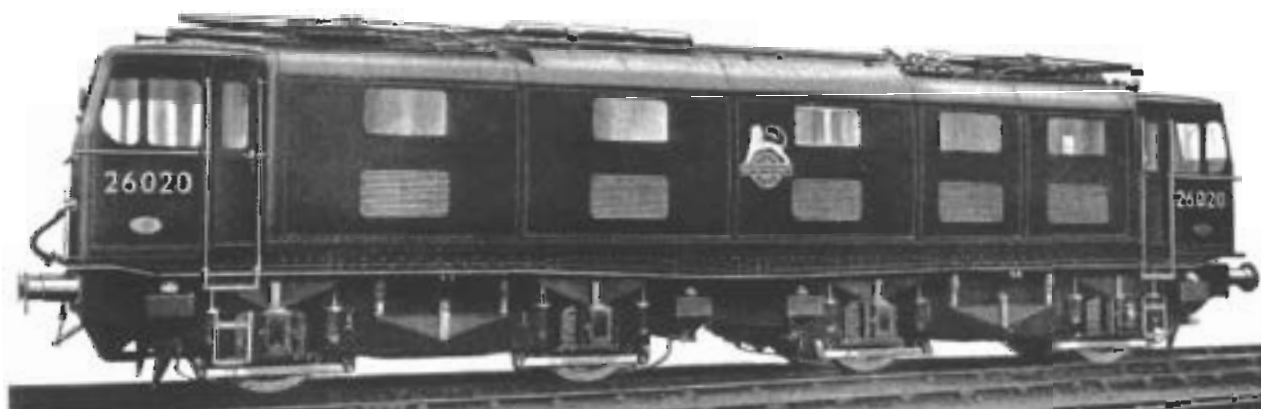
An 1868-hp four-axle Bo+Bo electric locomotive
